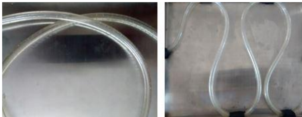
Fig 4: a) Porous tube used in the reactor b) Thin film bubbling reactor without the reactants
