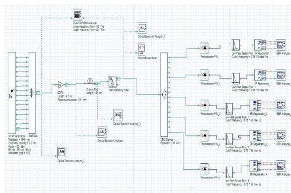
Figure 10: Schematic design of 16-channel WDM system, with introduction of Gain Flattening Filter (GFF).
