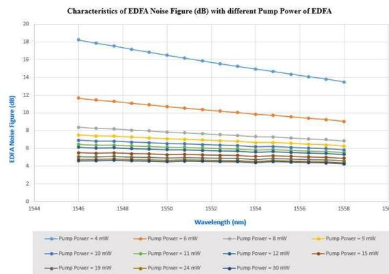
Figure 6: EDFA noise figure (NF) characteristics with various pump powers.
