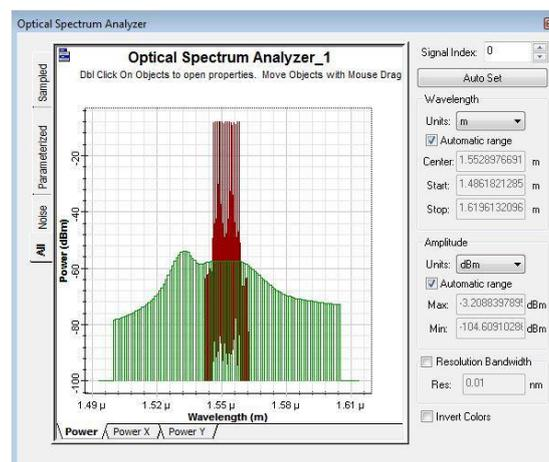
Figure 12: Flat output optical power spectrum (after GFF optimization).
