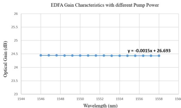
**Figure 16: Slope of gain characteristics w.r.t wavelength, while WDM system is re-configured with Hybrid Optical Amplifier (HOA).**
