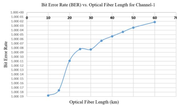
Figure 9: Characteristics of Bit Error Rate (BER) w.r.t optical fiber length for channel-1.
