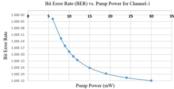
Figure 8: Characteristics of Bit Error Rate (BER) w.r.t EDFA pump power for channel-1.
