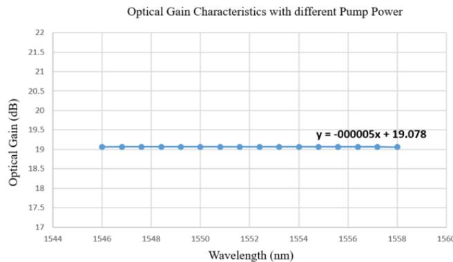
**Figure 14:** Slope of gain characteristics w.r.t wavelength, while the WDM is optimized with GFF.
