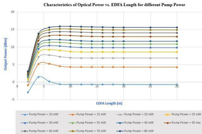
**Figure 3: Characteristics of output optical power vs. EDFA length for different pump power.**
