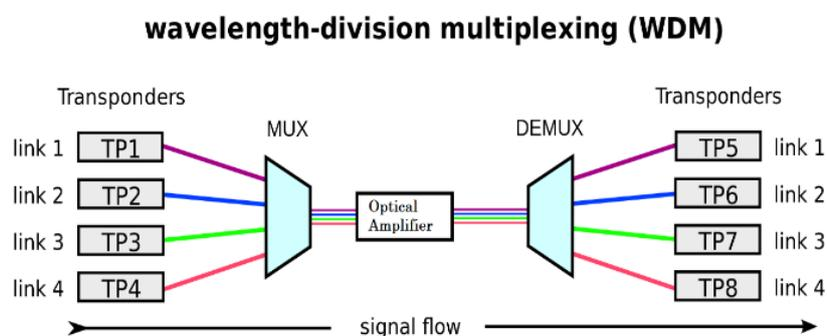
**Figure 1: Basic block-diagram of a typical WDM system.**
