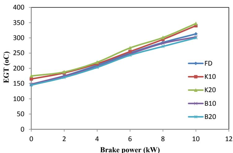
**Figure 5:** Variation of EGT with brake power.
