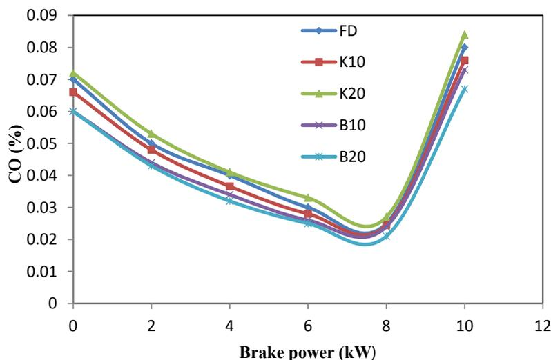
**Figure 6:** Variation of CO emission with brake power.
