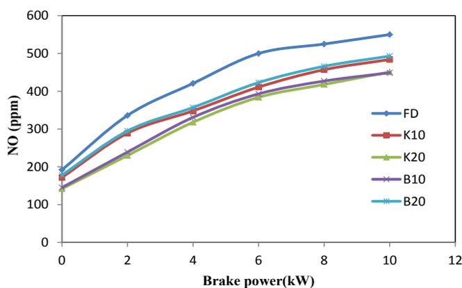
**Figure 8:** Variation of NO emission with brake power.
