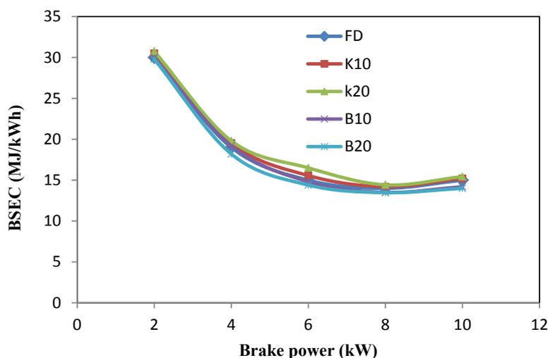
**Figure 3:** Variation of BSEC with brake power.
