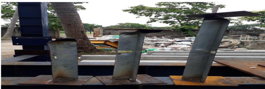
Figure 1. Angle sections of 400 mm, 500 mm and 600 mm lengths.
