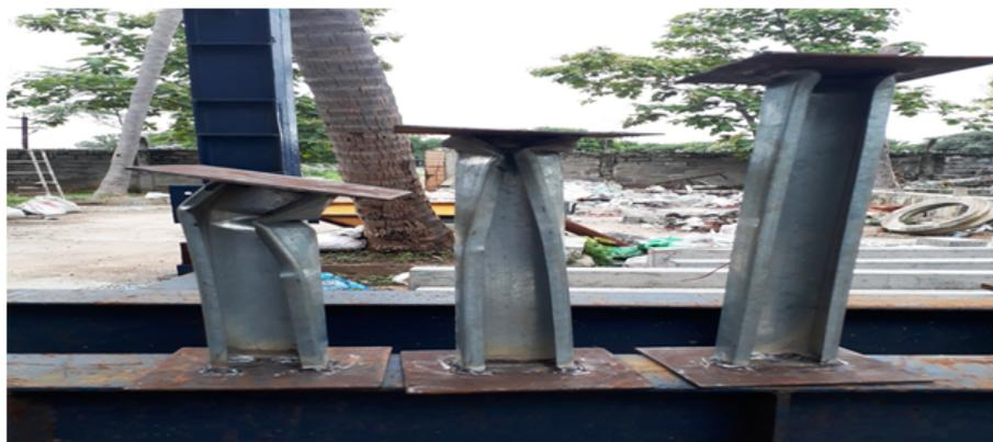
Figure 2: Channel sections of 400 mm, 500 mm and 600 mm lengths.
