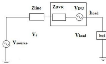
Fig. 2 Equivalent Circuit of DVR
