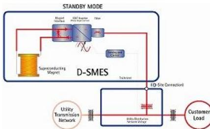
Fig. 3 Schematic diagram of SMES
