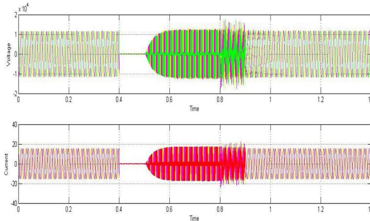
Fig. 8 Simulation results with SMES based DVR
