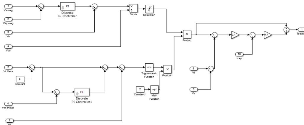
Fig. 5 Control block diagram of mitigation of fault current
