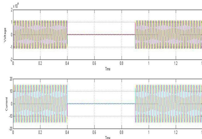
Fig. 7 Simulation results without DVR
