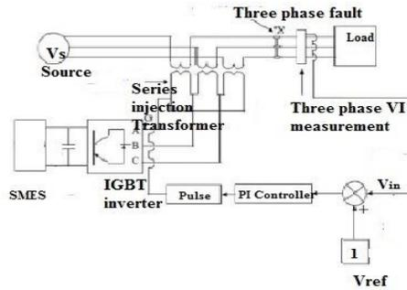
Fig. 4 Schematic diagram of SMES based DVR
