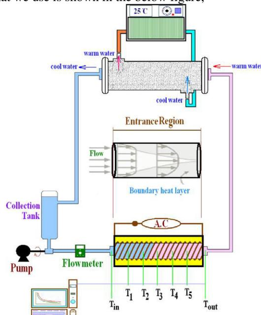
**Fig 2.2** schematic diagram of shell and tube heat exchanger
