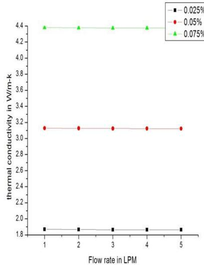
**Figure 3.1** thermal conductivity vs. flow rate
