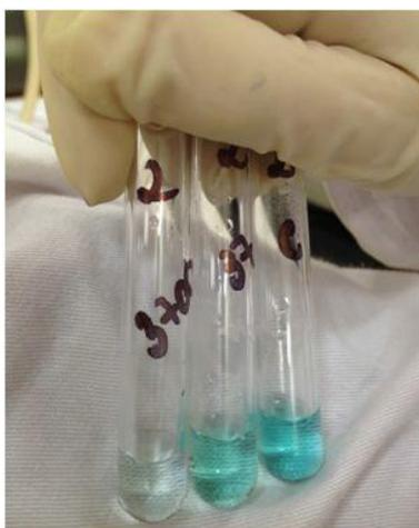
**Fig. 2.** Colors obtained by concentrations of 3700 ppm, 37 ppm and control.
