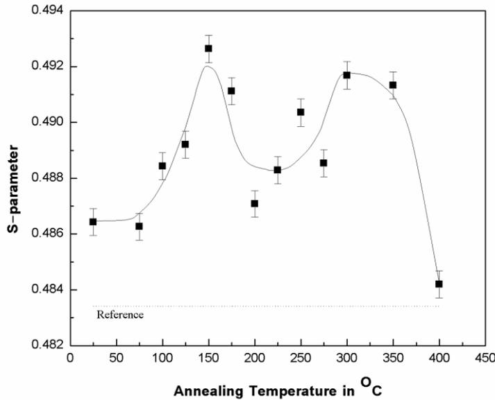
Fig. 1 Variation of S-parameter with annealing temperature in alpha irradiated undoped InSb. The dotted line is for unirradiated reference InSb sample.
