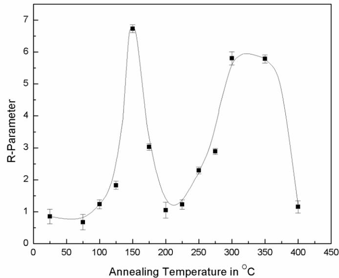
Fig. 2 Variation of R-parameter with annealing temperature in alpha irradiated undoped InSb.
