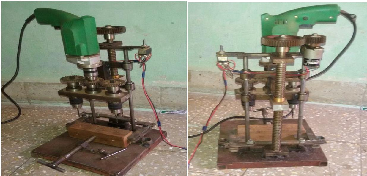
Fig 7.1 assembly of Twin drill head with depth control machine
