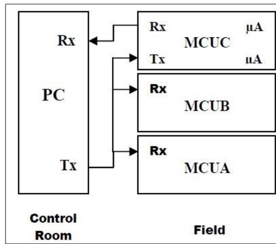
Fig. 5. Field controller schematic.
