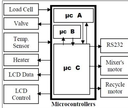
Fig. 7. Microcontrollers schematic.
