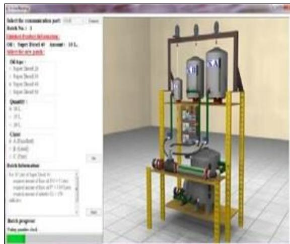
Fig. 8. Running program HMI.
