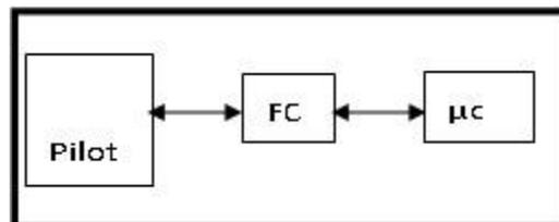
Fig. 4. Suggested control systems block diagram, FC: Field Controller, and  $\mu$ c: Main Controller" Laptop".
