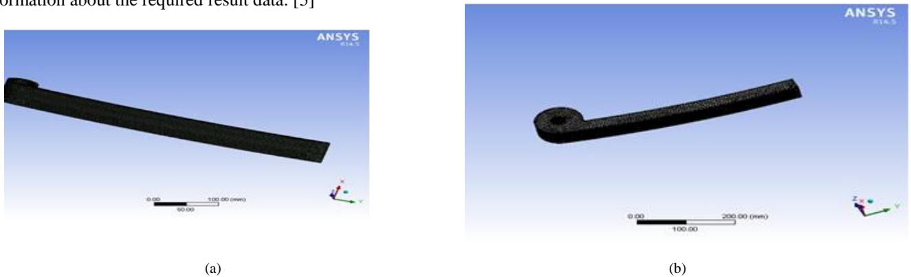
Fig. 2 Meshing of Leaf spring in ANSYS 14.5 (a) Meshing of Leaf Spring, Material EN47 steel (b) Meshing of Leaf Spring, Material: E Glass/Epoxy
