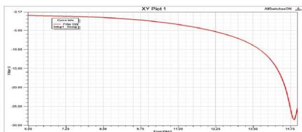
Fig.5.Simulated returnloss of the antenna with filter in OFF state
