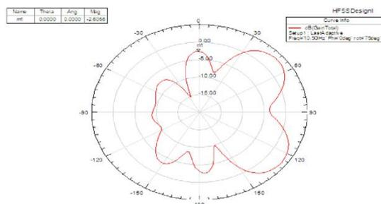
Fig.6. Normalized radiation pattern of the UWB antenna when Filter is in OFF state.
