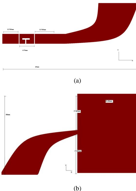
Fig.2. Simulated structure of antenna (a) Top layer (b) Bottom Layer with dimensions in mm.
