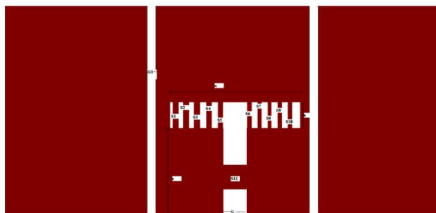
Fig.1: Defected Microstrip Structure (DMS) Filter with a=2.9mm, b=0.8mm, c=2mm, g=0.25mm, g1=0.2mm with S1, S2, S3, S4, S5, S6, S7, S8, S9, S10 and S11 switches.
