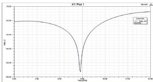
Fig.4.Simulated returnloss of the antenna with filter is ON
