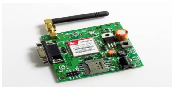
Fig.5 GSM Modem (SIM900)
