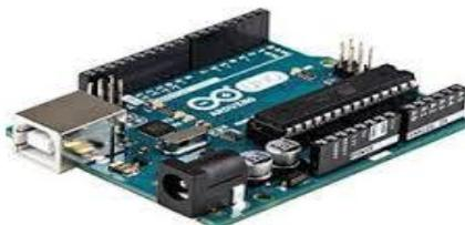
Fig.3 Arduino UNO development board
