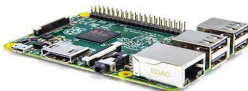
Fig.2. Raspberry pi2 model B.
