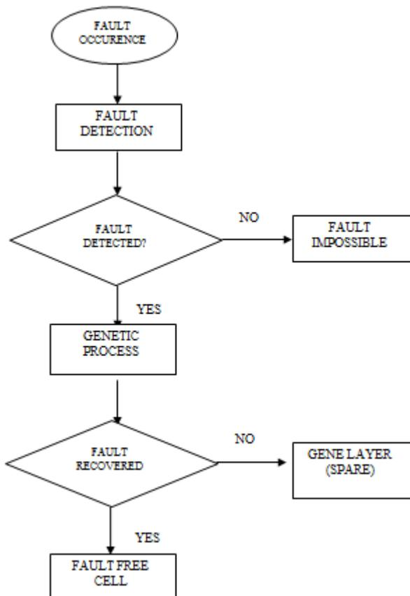
Fig .3 Fault detection and Correction
