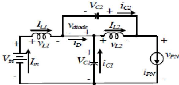
Fig. 5. Equivalent circuit of qZSI in active mode
