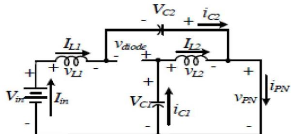
Fig. 6. Equivalent circuit of qZSI in shoot through mode
