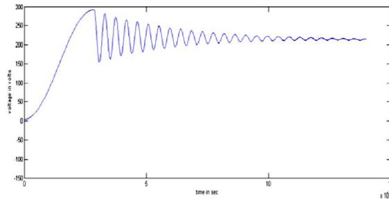
Fig. 11. Quasi Z-Source Inverter Output Voltage
