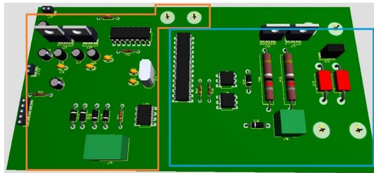
**Figure 2:** Orange box represents the step of sensing and the blue box the rectifier circuit.
