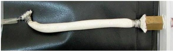
Fig. 4 Pneumatic Artificial Muscle [19]
