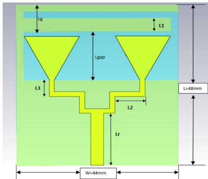
Fig.2 GEOMETRY OF ANTENNA WITH E-SHAPED DGS
