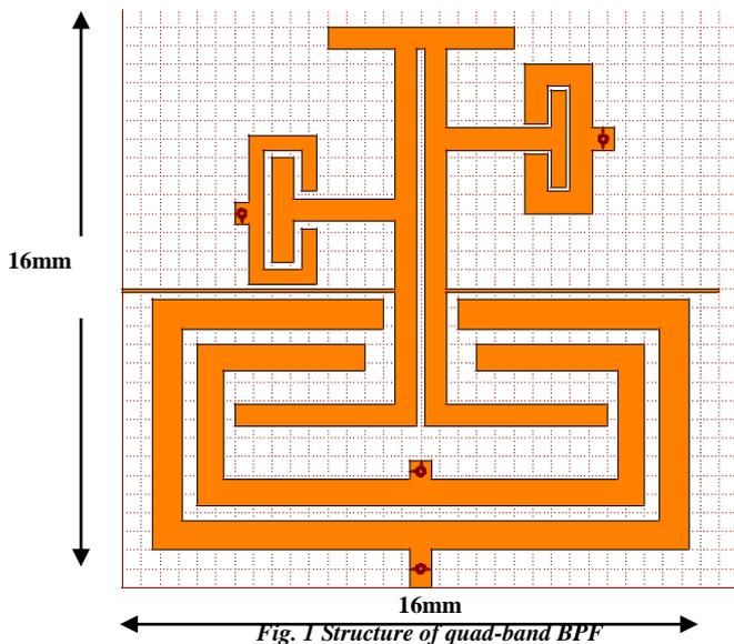
Any value of reactance can be made, as stub length is varied from zero to half a wavelength. Four shorted stubs are attached with each of the resonator. The stubs are shorted for the frequency selective operations over the LTE frequency bands. The size of the circuit is 16x16mm. FR4 is used as the substrate with 4.4 as dielectric constant ( $\epsilon_r$ ). The distance between the resonator and the feed line is 0.2mm.
