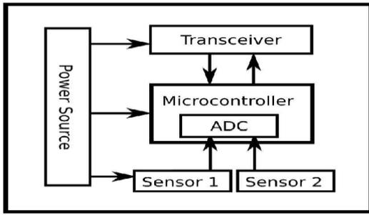
Block diagram of a Wireless Sensor Node
