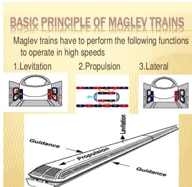
**Figure 1 Basic Principle In Maglev Trains**
