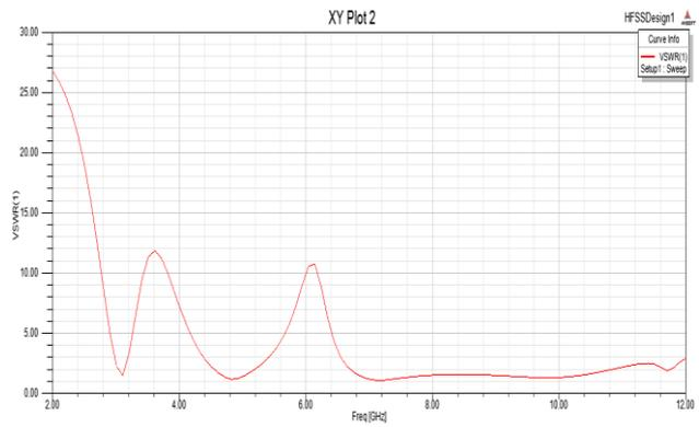
Fig.4 simulated VSWR characteristics of the antenna
