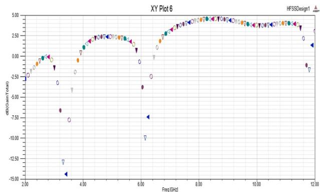
Fig.5 simulated gain of the designed antenna
