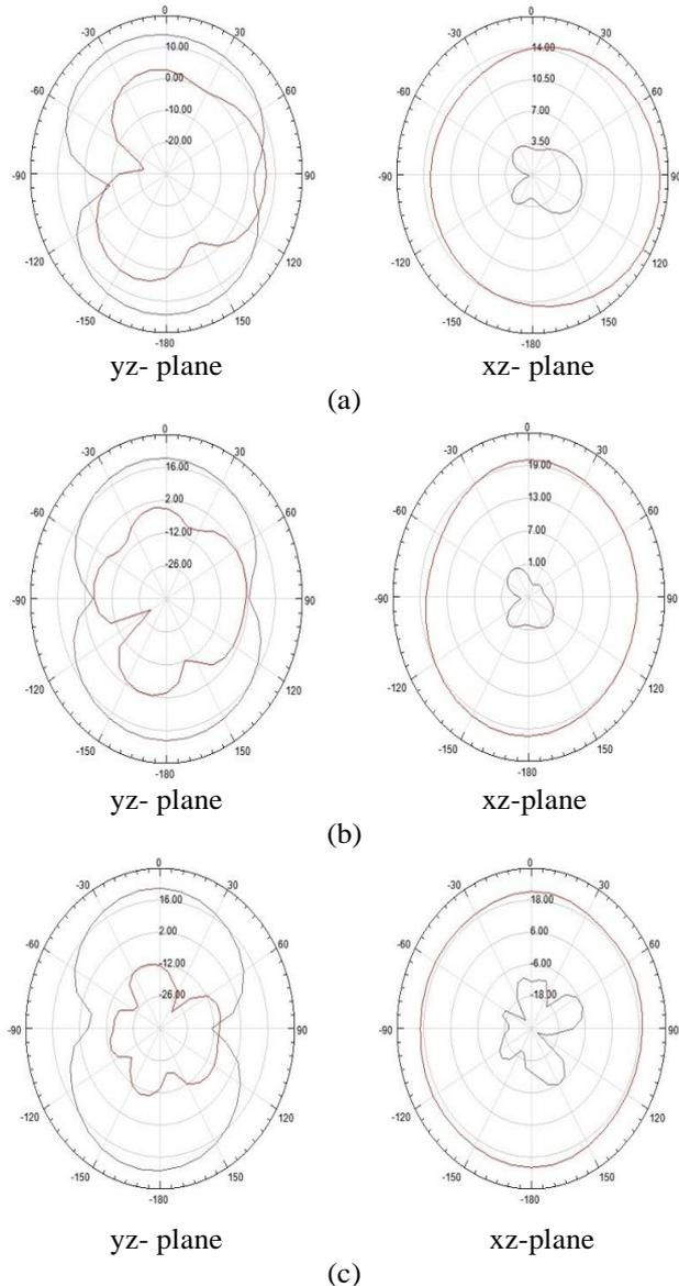
Fig.6 Radiation patterns of the antenna. (a).3.1GHz, (b).4.8GHz and (c) 7.2 GHz.
