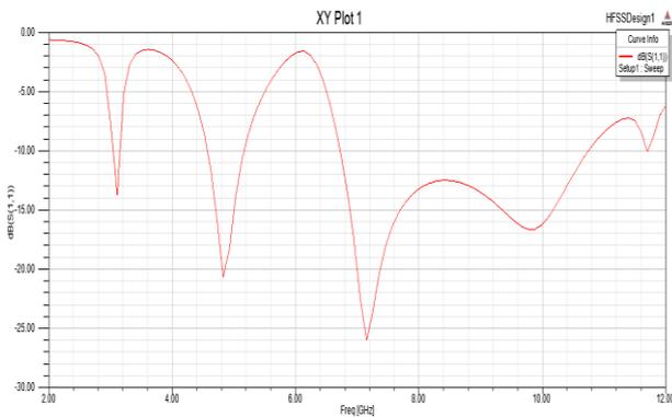
Fig.3 simulated S-parameter of the antenna
