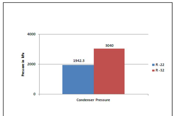
The operating pressures of R-32 are 45.78 % higher at evaporator and at condenser it is 56.5 % higher than that of R-22. As R-32 is an eco friendly refrigerant, it can be used in RAC systems, by altering the manufacturing process, so as to get sufficient strength to withstand high operating pressures.
