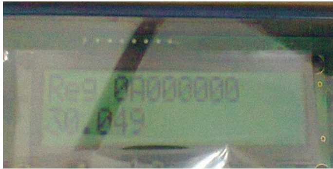
Fig. 1. Temperature value displayed in meter LCD
