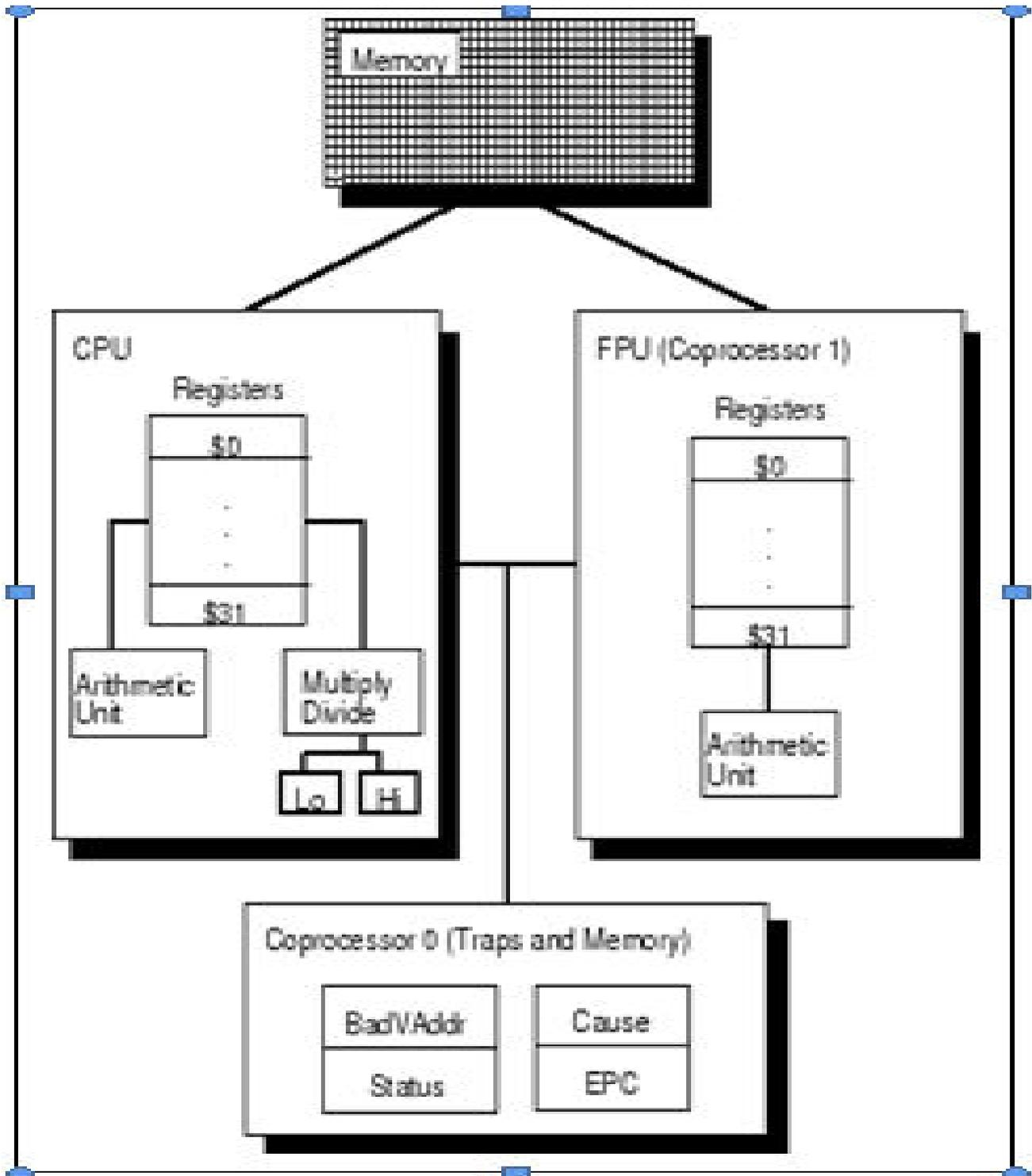
Fig.1. Block Diagram of MIPS R2000
