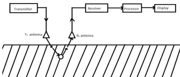
Fig2: Ground Penetrating Radar block diagram.
