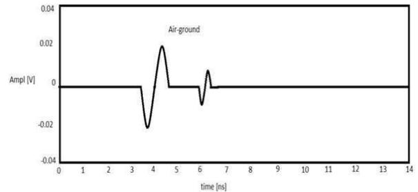
Fig3: Typical signal, received by the GPR
