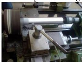
Fig. 2(a) Turning operation
