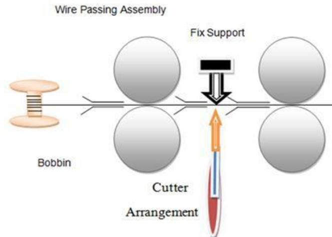
**Figure 6: Block diagram of proposed system top view.**
