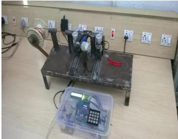
**Figure 8: Automatic wire cutting system.**
