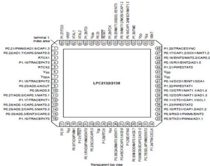
Figure 1: Pin diagram LPC 2138.
