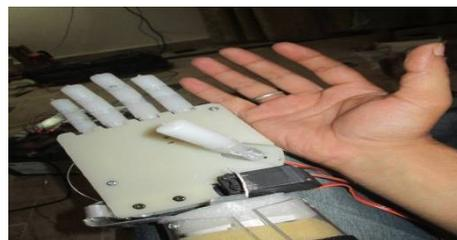
Fig.9. Depicting a Myoelectric prosthetic hand designed
