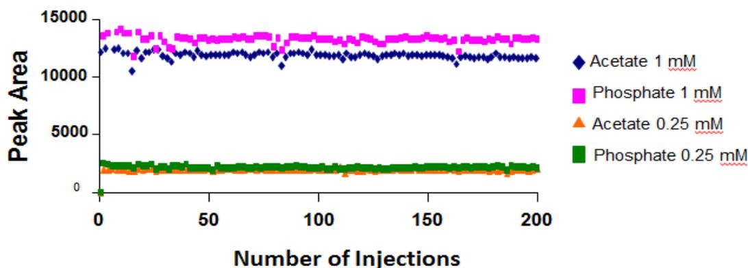
**Figure 5B.** Alternating injection between 0.25 mM (100 injections) and 1 mM (100 injections) acetate and phosphate standards to evaluate peak area precision of total 200 injections. The peak area % RSD is  $<5\%$  at 0.25 mM and  $<3\%$  at 1 mM acetate and phosphate concentration.
