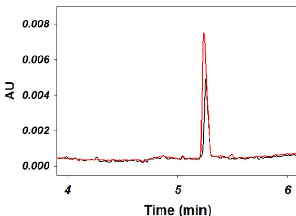
**Figure 4B.** 0.25 mM phosphate standard was spiked into 40x diluted D2 step sample showing peak at 5.2 min increases.
