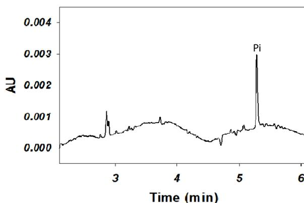
**Figure 2C.** Electropherogram of the same D2 step sample with 40x dilution to analyze the phosphate.
