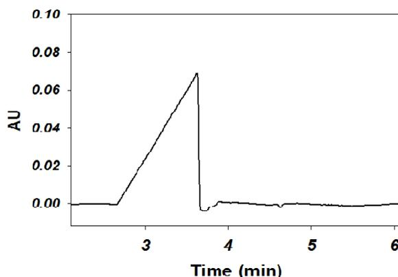
**Figure 2D.** Electropherogram profile of final aqueous product (FAP) sample illustrating the absence of acetate and phosphate peaks. The large chloride peak observed from 2.5 min to 3.5 min is attributed to the presence of NaCl in FAP sample.
