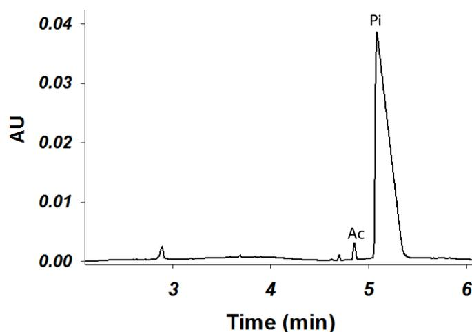
**Figure 2B.** Electropherogram of D2 step sample injected neat showing acetate peak at about 4.8 min and large phosphate peak at about 5.2 min.
