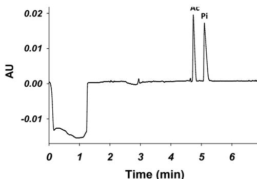
**Figure 1.** An electropherogram of standard acetate (Ac) and phosphate (Pi) anions each injected at 1 mM. Their migration times are about 4.8 and 5.2 min, respectively.
