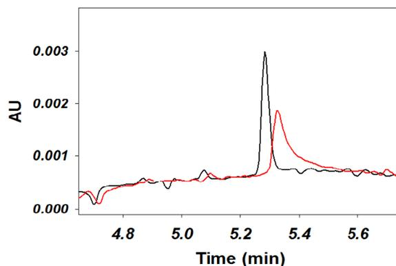
**Figure 3A.** The phosphate peak is shown at injection 1 (black trace) and peak tailing at injection 90 (red trace).
