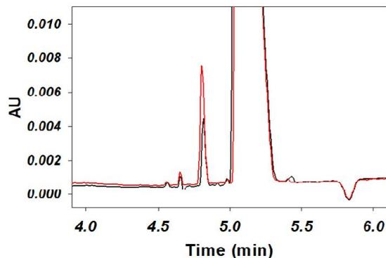
**Figure 4A.** Peak identity confirmation and spike recovery experiments (A) 0.25 mM acetate standard was spiked into D2 step sample showing peak at 4.8 min increases.
