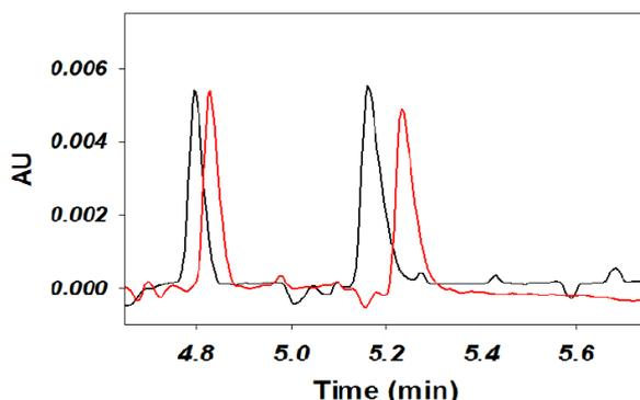
**Figure 3B.** Acetate and phosphate peaks in standard sample are shown at injection 1 (black trace) and injection 200 (red trace) without any peak tailing after increasing the NaOH and HBr washes to 3 min at the end of separation. The migration time shift is likely due buffer depletion.
