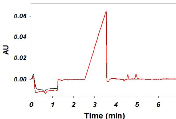
**Figure 4C.** : 0.25 mM acetate and phosphate standards were spiked into FAP sample.
