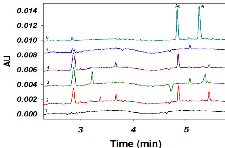
**Figure 2A.** Electropherograms of water injected from various filters screening; blank water without filter as control (trace 1), PALL 3K (Trace 2), YM30 (Trace 3), PALL 10K (Trace 4), and Millipore 30K (Trace 5). Trace 6 is acetate and phosphate standards that were filtered using Millipore 30K.
