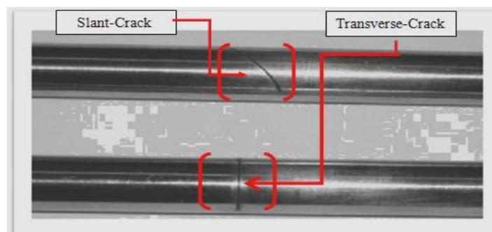
Fig. 1 Transverse-cracked shaft and slant-cracked shafts
