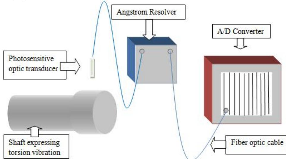
Fig. 1 Torsional vibration measurement instrumentation using a fiber optic probe approach
