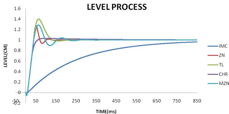
In figure 2, the calculated values are shown in the form of responses, where (A) is the open loop response used for the determination of transfer function, which is needed for the process differentiation. (B) is the outcome of the system function with different tuning techniques and it is also used for comparison that increases the chance of finding the best controller action for the given system.
