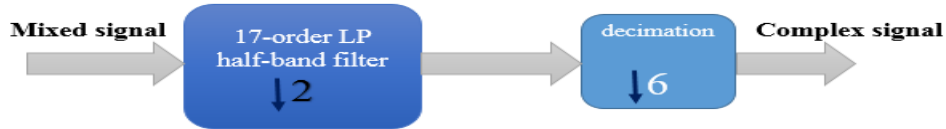
Figure 2. Modified filter structure
