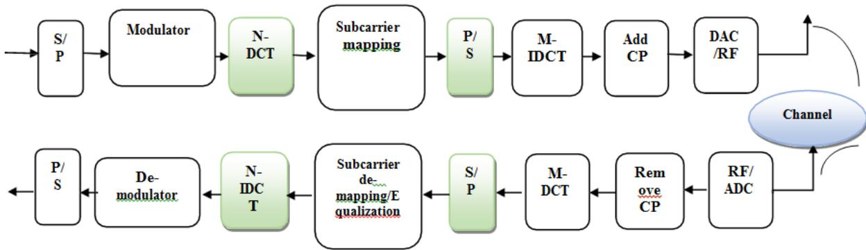
**Figure 3: block diagram of the DFT-SC-FDMA system.**
