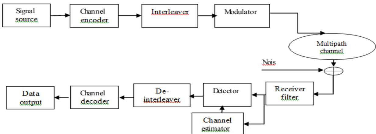
Figure 5: Block diagram for a system utilizing channel estimator and detection.
