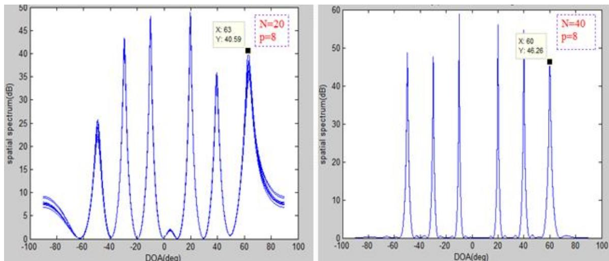
Figure4: Array pattern of coherent signals for varying number of elements
