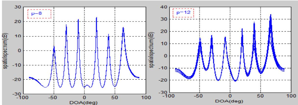
Figure 6: Array pattern versus the number of sub arrays
