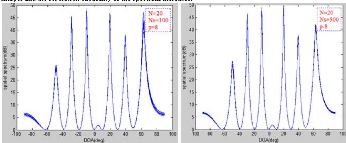
Figure5: Array pattern of coherent signals for varying number of snapshots
