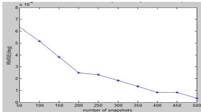
Figure 9 : RMSE curve of the DOA estimates with  $p = 2$  sub arrays versus the number of snapshots
