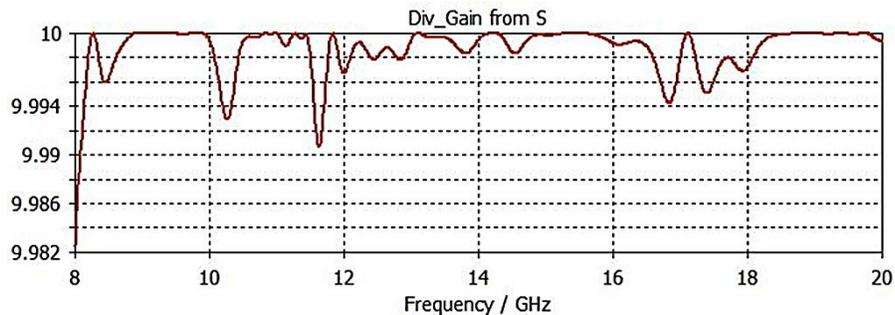
**Figure 7: Simulated diversity gain characteristics of the antenna.**
