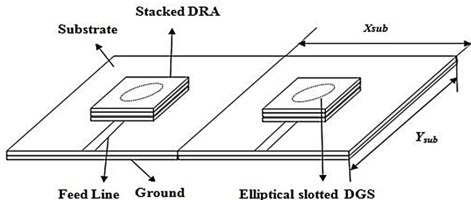
Figure 1: 3D view of geometry of the proposed 5G antenna.
