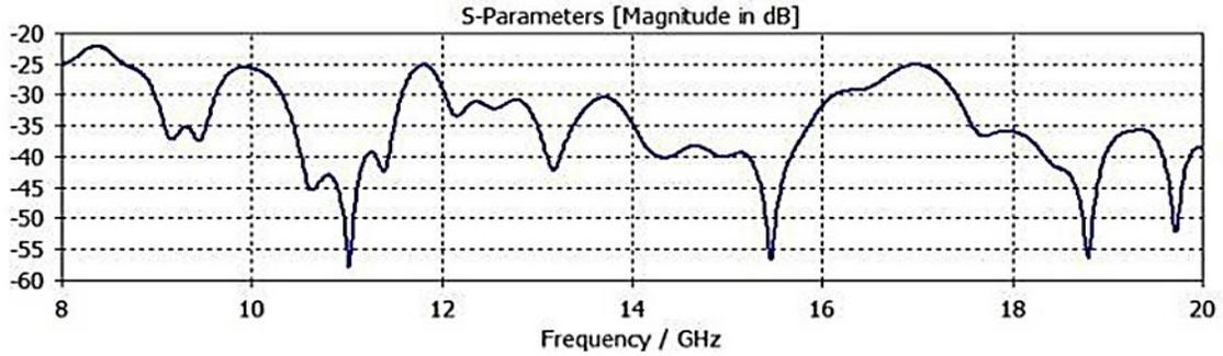
**Figure 3: Simulated reflection coefficient (S11) characteristics of antenna.**
