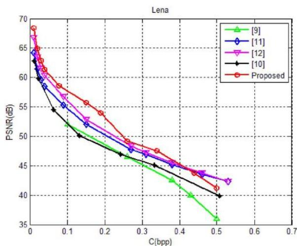
Fig. 3. Embedding capacity ( ) versus image distortion (PSNR) of our approach in comparison with the reversible schemes [9]–[12]. The test set is constituted of gray-scale image Lena
