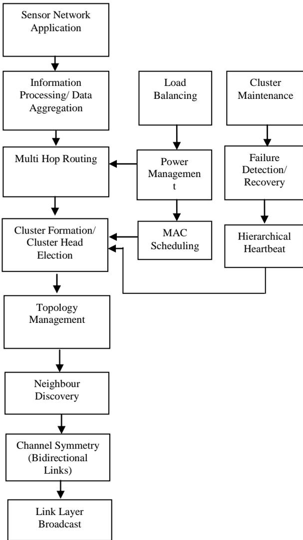
Fig. 3. Depends-on hierarchy for cluster-based sensor network routing protocols. The function at the tail of an arrow depends on the function at the head of the arrow.
