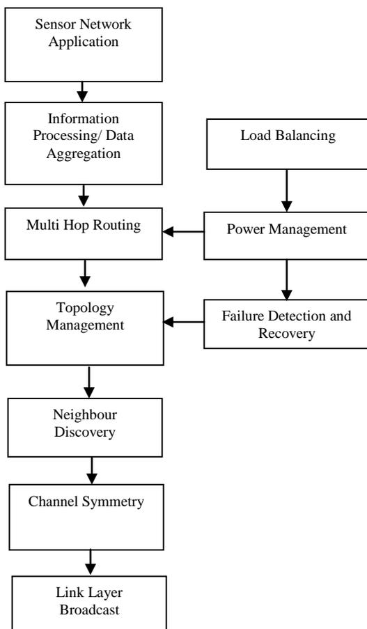
Fig. 2. Depends-on hierarchy for flat sensor network routing protocols. The function at the tail of an arrow depends on the function at the head of the arrow
