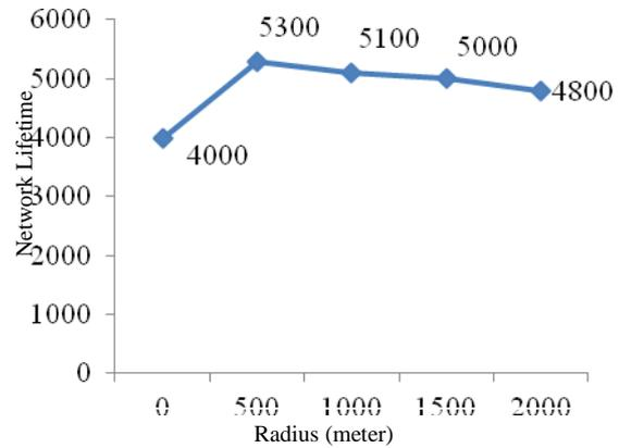
Fig. 6 Effect of hybrid boundary on network lifetime.
