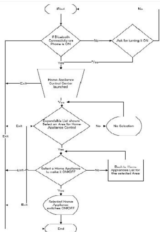
Fig 3. Flow Chart: Android Mobile Application Program
