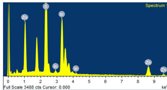
**Fig.7** EDAX Spectrum of the as-deposited ZnIn<sub>2</sub>S<sub>4</sub> (ZIS) thin film
