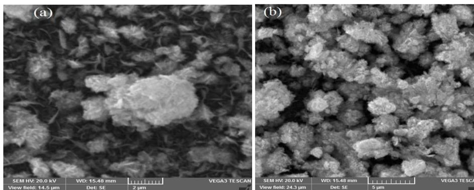
**Fig.8** FESEM as-deposited ZnIn<sub>2</sub>S<sub>4</sub> (ZIS) thin film with different magnification such as (a) 2 μm, (b) 5 μm.
