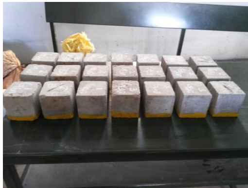
Fig.2. Specimens for sorptivity test
