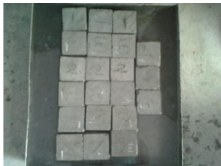
Fig.1. Specimens during water absorption test
