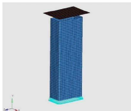
Fig.4 Meshed model of rectangular tube
