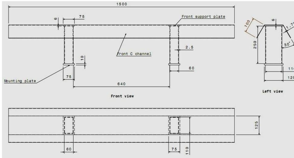
Fig.7 Orthographic View of Bumper System
