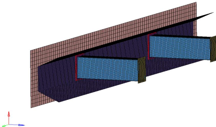
Fig.6.Modelling of bumper System
