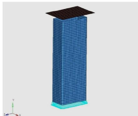
Fig.4 Meshed model of rectangular tube
