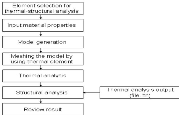
Figure 2. Flow chart for analysis procedure
