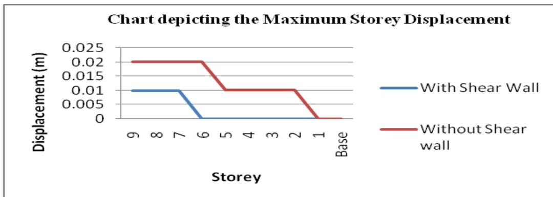
**Fig. 4.10 Chart showing Maximum Storey Displacement**
