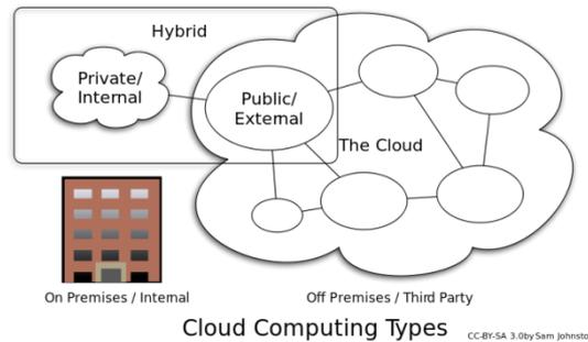
Figure 3.2: Cloud Deployment Model
