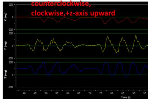
Figure 10: iNEMO test signal(counterclockwise, clockwise,+z-axis upward).
