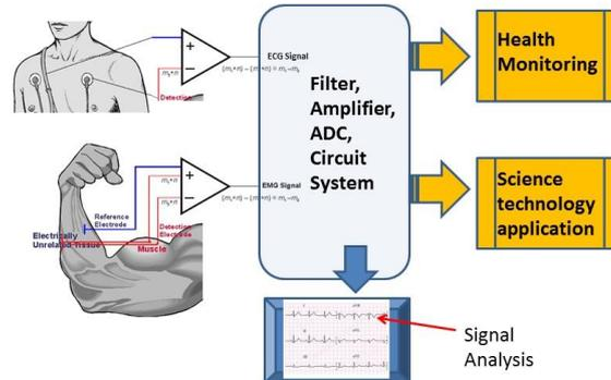
**Figure 3:** The Electrocardiogram (ECG) and electro myogram (EMG) signal capture system.
