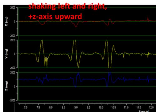
**Figure 9:** iNEMO test signal (shaking left and right, +z-axis upward).
