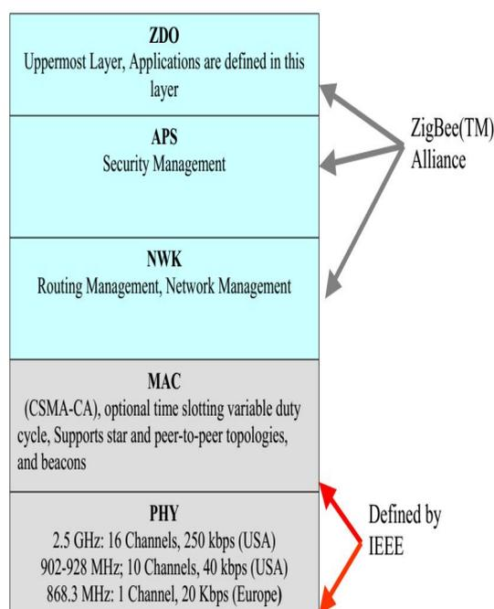
Figure 2. ZigBee(TM) Stack
