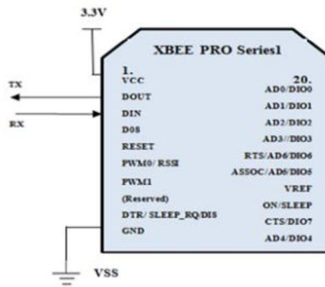
Figure 4: Schematic diagram for XBEE
