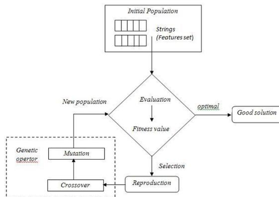
Fig. 3. Genetic Algorithm - A Flowchart
