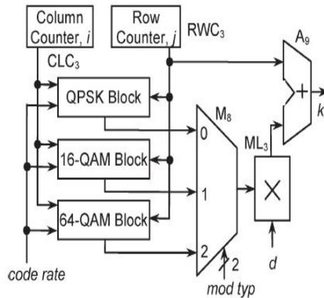
Fig3: Proposed deinterleaver architecture
