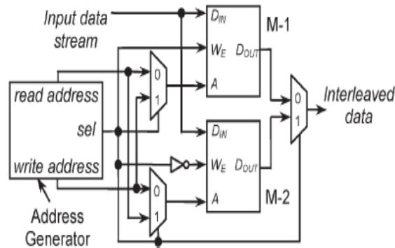
Fig2. Deinterleaver Architecture
