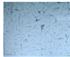
Fig-2 Microstructure for defect free casting
